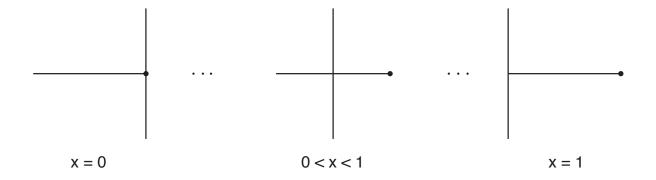
A century earlier, Franz Reuleaux used the same method for machinery, to classify the forms of a nut and bolt in terms of the pitch-angle  $\theta$  of the screw – the standard twisting pairs with helical motion are flanked at 0 by a turning pair with rotary motion, an axle and wheel, and at  $\pi/2$  by a sliding pair with translational motion on a linear track. For Reuleaux, it goes like so –
