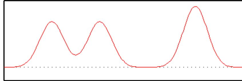
Try to represent this function in terms of sine waves. The first sine wave has a frequency of 2, that is there are two repeats of the wave across the unit cell. One peak represents the oxygen, and the other the two carbons:
