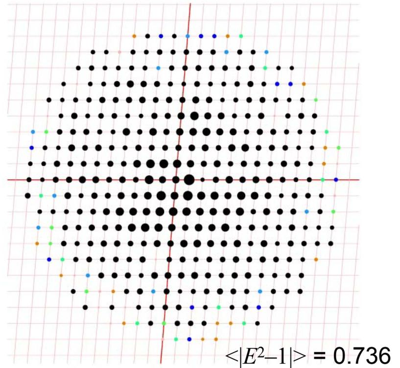
$2kl$  projection of the reflections of a structure in the space group  $P1$ .
