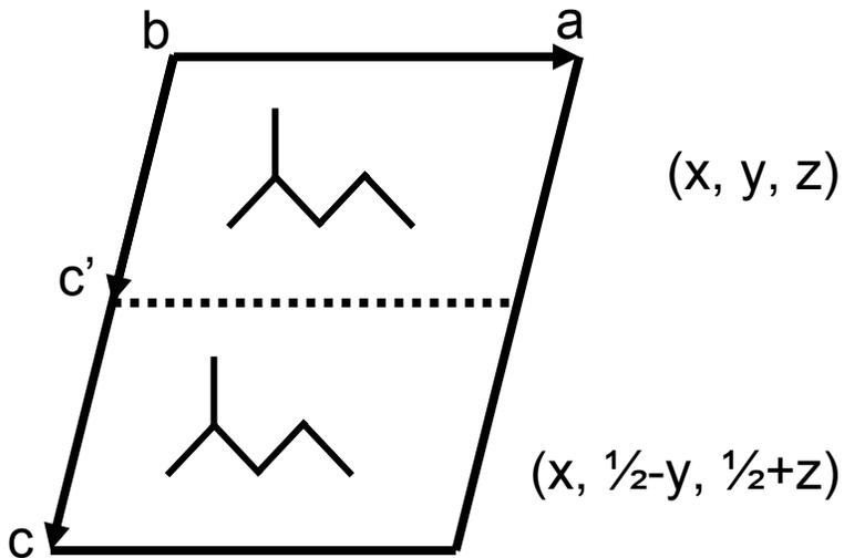
In this two 2D projection the structure is repeated at  $c/2$ . Thus, the unit cell seems to be half the size:  $c' = c/2$  in this projection.
