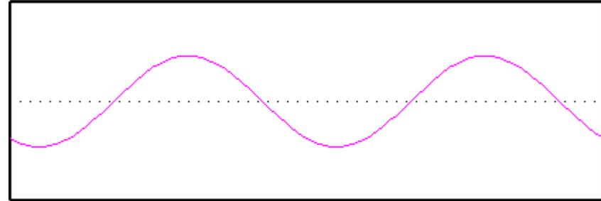
The second sine wave has a frequency of 3; three repeats of the wave across the unit cell. It has a different phase, in other words we start at a different place on the wave. The amplitude is also different:
