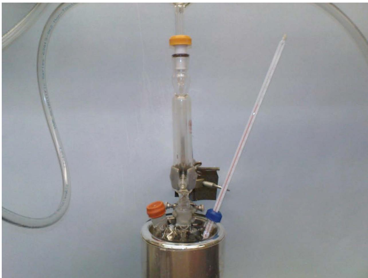
**Figure 3. Set up for the in situ generation of the CAB catalyst and Diels-Alder reaction.**
