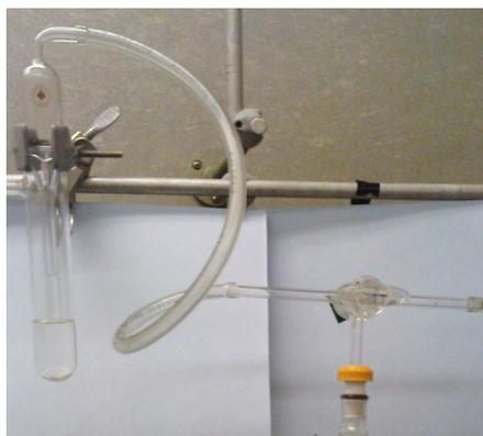
**Figure 1. Reaction setup for the esterification reaction.**
