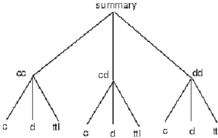
**Figure 1:** Example of the summary data structure, as a tree. The top level has three pieces, corresponding to the actions of the other players (both cooperated, only one cooperated, both defected). The second level has three pieces, listing the number of times the player cooperated, defected and the total number of times the situation specified by the actions of the opponents occurred.
