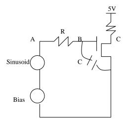
As the frequency is increased, the capacitance at the gate acts more as a short. Thus the MOSFET has a smaller input, resulting in a smaller output.
