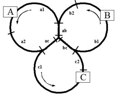
With this setup, each of Alice, Bobby, and Chip have their own trains, and each train travels in a circular path in the indicated (counterclockwise) direction. Note that there is a section of track shared between each pair of trains. In order to avoid sibling battles due to train wrecks, Gill has devised a system for segmenting the track, and has programmed each train to use a semaphore to avoid simultaneous use of the shared track sections **ac**, **ab**, and **bc**.
