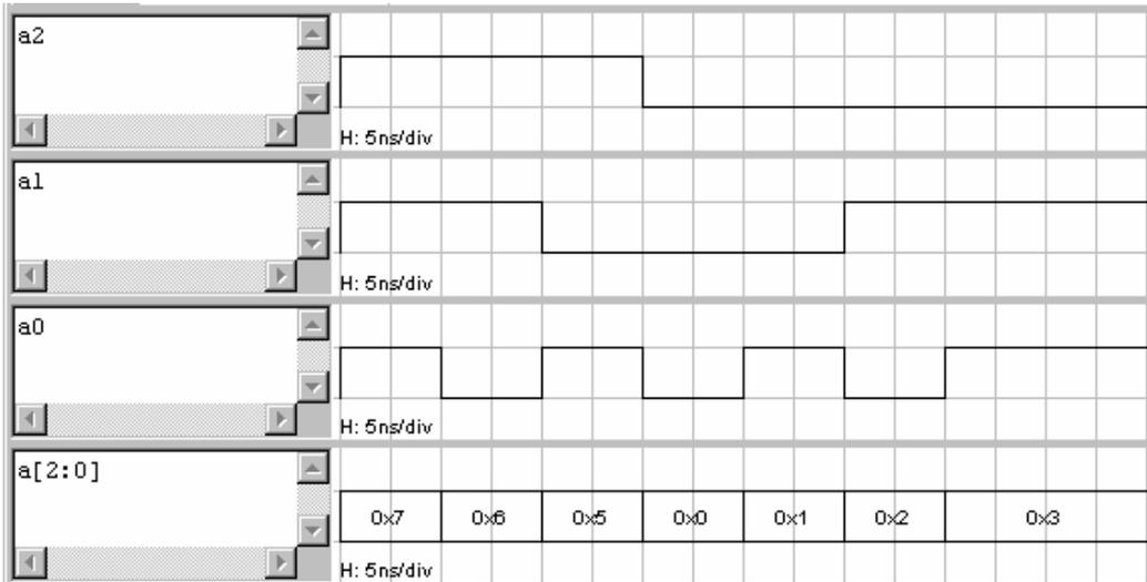
JSim knows how to plot a set of nodes as a single multi-bit data value, as shown in the bottom channel of the plot above. If you zoomed in on one of the transition times, you would see that the values actually turn to “X” for 0.1ns while making the transition between valid logic levels.
