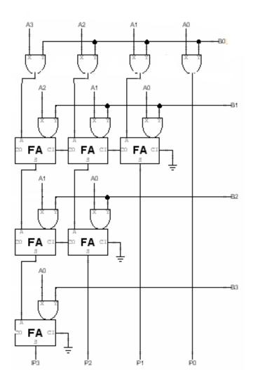
The circuit above works with both unsigned operands and signed two's complement operands. This may seem strange – don't we have to worry about the most significant bit (MSB) of the operands? With unsigned operands the MSB has a weight of  $2^{\text{MSB}}$  (assuming the bits are numbered 0 to MSB) but with signed operands the MSB has a weight of  $-2^{\text{MSB}}$ . Doesn't our circuitry need to take that into account?
