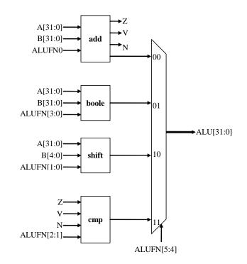
Two additional control signals (ALUFN[5:4]) have been introduced to select which unit will supply the value for the ALU output. The encodings for ALUFN[5:0] used by the test jig are shown in the following table:
