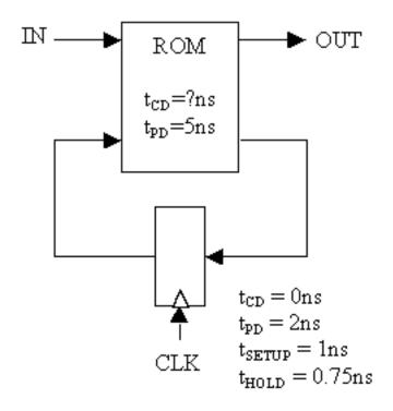
A. What is the smallest value for the ROM's contamination delay that ensures the necessary timing specifications are met?
