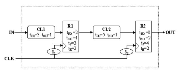
D. Rewrite the timing specifications for the system as a whole taking into account d1 and d2. Don't
