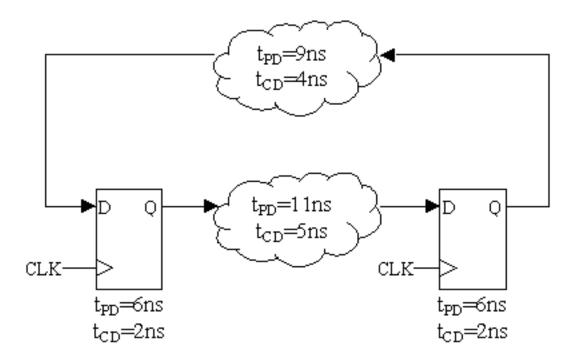
C. Assuming that the clock period is 25ns, what is the maximum setup time for the flip-flops for which this circuit will operate correctly?
