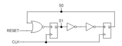
inverter: t<sub>CD</sub>=1ns, t<sub>PD</sub>=2ns nor2: t<sub>CD</sub>=1.5ns, t<sub>PD</sub>=2ns D register: t<sub>CD</sub>=0ns, t<sub>PD</sub>=2ns, t<sub>H</sub>=1ns, t<sub>S</sub>=3ns
