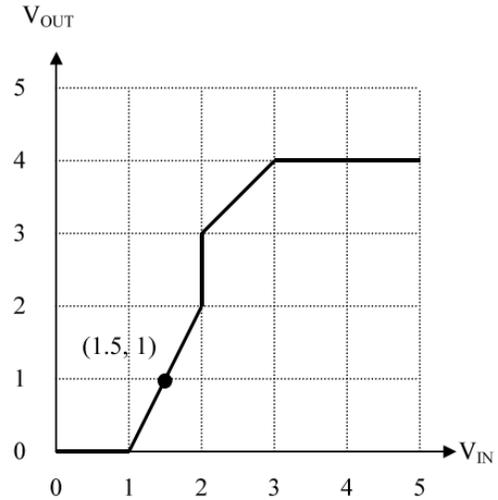
Your job is to choose a single set of signaling thresholds  $V_{ol}$ ,  $V_{il}$ ,  $V_{oh}$ , and  $V_{ih}$  to be used with both devices to give the best noise margins you can. Recall that the VTC can touch the edge of the forbidden regions but not pass through those regions. Fill in your answers below, together with the resulting noise margins. You'll get partial credit for anything that works with nonzero noise margins; for full credit, maximize each of the noise margins.
