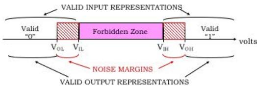
A combinational device accepts marginal inputs and provides unquestionable outputs (to leave room for noise).
