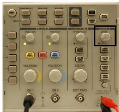
Figure 7: The “LEVEL” knob sets the trigger level.
