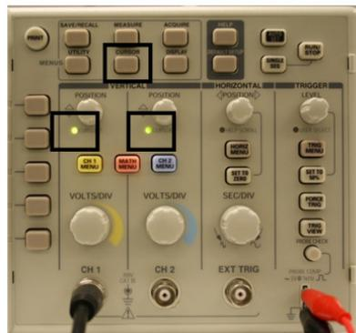
Figure 9: The “CURSOR” button toggles the Cursor Mode. When the LEDs are lit, that means you are in Cursor Mode, and the “POSITION” knob now controls the cursor.
