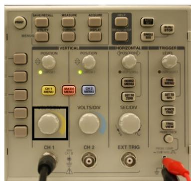
Figure 4: The “VOLTS/DIV” knob that scales the Y-axis.
