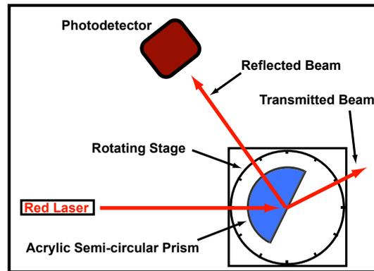
Figure 2: Setup to measure Fresnel coefficient
