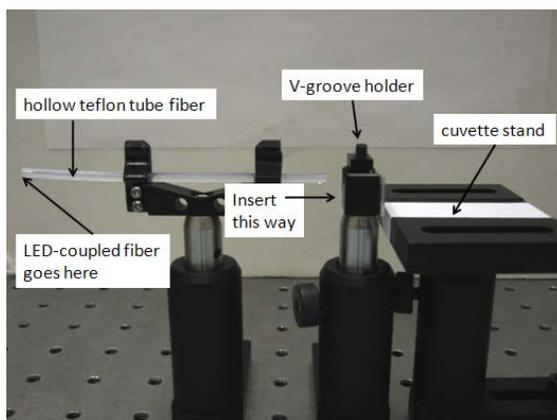
Figure 3: Setup for holding the hollow tube fiber.
