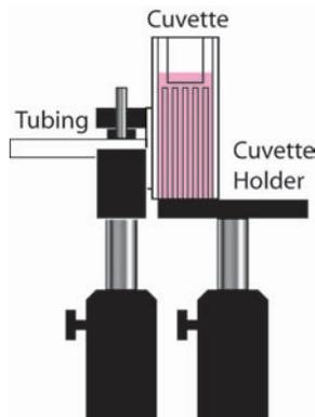
Figure 7: Illustration of the spectrometer configuration for measuring the cuvette.
