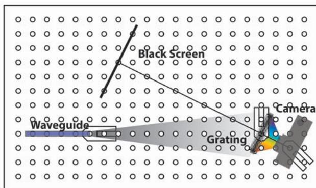
Figure 4: Schematic for building the spectrometer.
