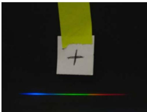
Figure 5: Camera image of an aligned spectrometer.
