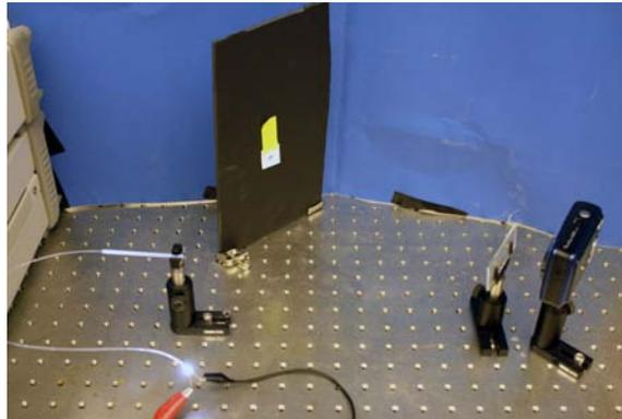
Figure 6: Image of the spectrometer setup on the optical table.
