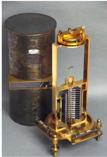
Figure 5.2.1: Example of electrostatic voltmeter.
