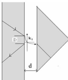
Figure 1: Schematic of frustrated internal reflection.
