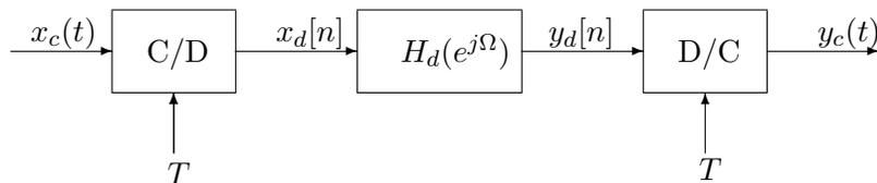
The C/D converter samples its input at integer multiples of  $T$ :
