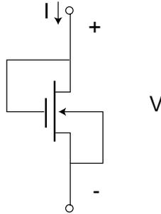
(3a) (10 points) In terms of usual MOSFET parameters, derive suitable equations for the I-V characteristics of the resulting two-terminal device. Sketch the I-V characteristics in a linear scale.
