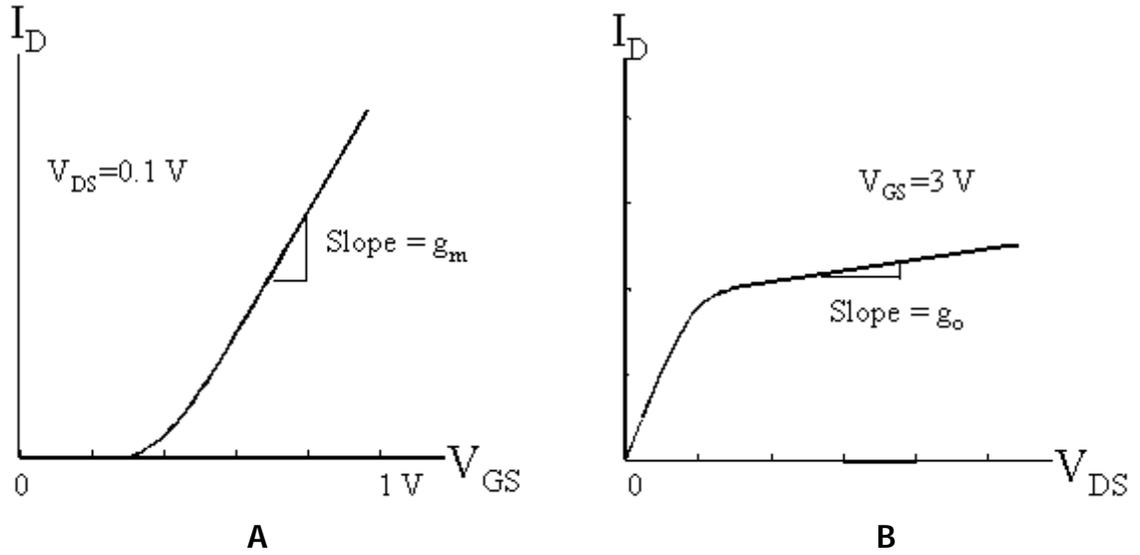
In (A),  $g_m = 1.4 \times 10^{-4} \text{ A/V}$ . In (B),  $g_o = 5.7 \times 10^{-5} \text{ A/V}$ .
