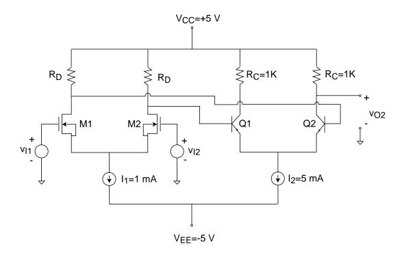
M1 and M2 are identical and are biased in the saturation regime. Q1 and Q2 are also identical and are biased in the forward active regime. Suitable parameters for these transistors are:
