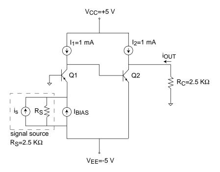
Both transistors in this amplifier are identical and are characterized by the following parameters:  $\beta_F = 100$  and  $V_A = 50 V$ . Treat all biasing current sources as ideal, that is, with infinite internal resistance.
