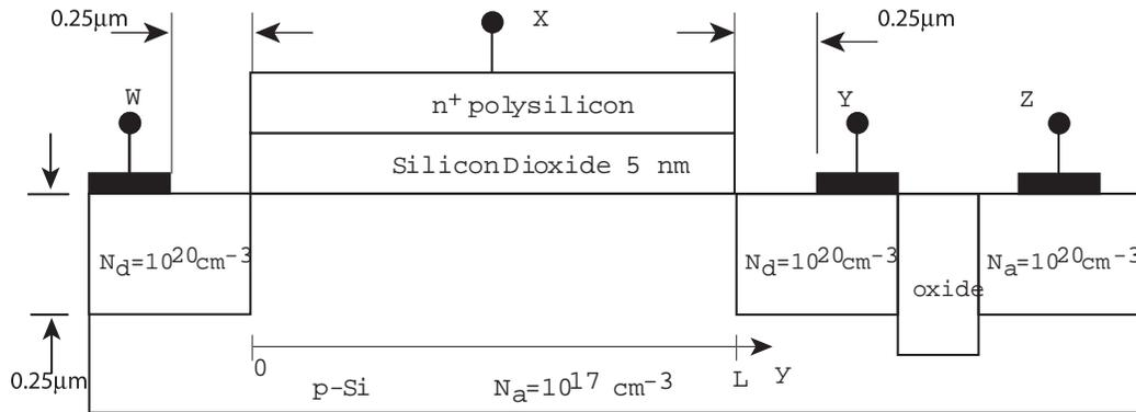
(2a) (4 points) If the device is to be operated as an n-channel MOSFET, identify the terminals (answer W, X, Y, or Z in the space provided below):
