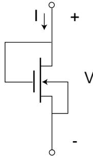
Derive suitable equations for the I-V characteristics of the "diode",  $I$  vs.  $V$  for  $V < V_T$ , and  $V > V_T$ . Sketch the I-V characteristics in a linear scale.
