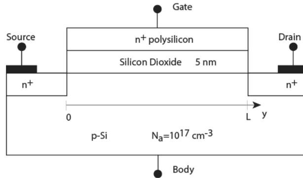
A capacitance voltage curve of the  $n^+$  poly-silicon gate MOSFET was taken by connecting the source, drain and body terminals together. A voltage was applied between the gate and the body.
