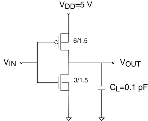
In the above diagram, the two numbers next to each transistor give its gate dimensions (width/length) in microns. In solving this problem, assume that  $C_L$  is the dominant capacitance in this circuit. All other capacitances can be neglected next to  $C_L$ .
