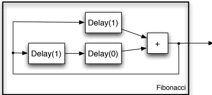
**Figure 4.8** Machine to generate the Fibonacci sequence.
