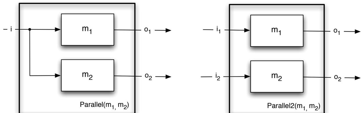
**Figure 4.5** Parallel and Parallel2 compositions of state machines.
