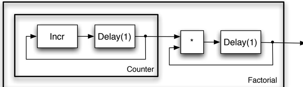
**Figure 4.9** Machine to generate the Factorial sequence.
