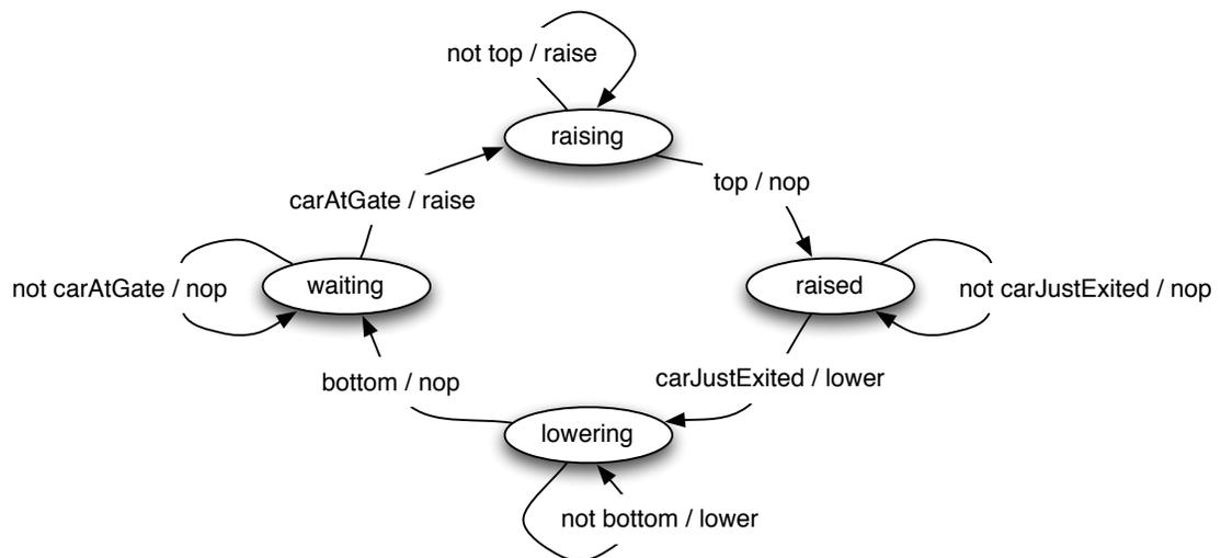
**Figure 4.3** State transition diagram for parking gate controller.
