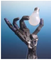
Courtesy of the Shadow Robot Company. Used with permission. Shadow Dexterous Robot Hand (Greenhill and Elias)
