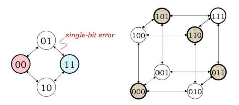
Figure 5-2: Codewords separated by a Hamming distance of 2 can be used to detect single bit errors. The codewords are shaded in each picture. The picture on the left is a (2,1) repetition code, which maps 1-bit messages to 2-bit codewords. The code on the right is a (3,2) code, which maps 2-bit messages to 3-bit codewords.
