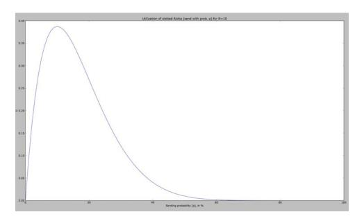
Figure 15-3: The utilization of slotted Aloha as a function of p for N = 10. The maximum occurs at p = 1/N and the maximum utilization is  $U = (1 - \frac{1}{N})^{N-1}$ . As  $N \to \infty$ ,  $U \to \frac{1}{e} \approx 37\%$ . N doesn't have to be particularly large for the 1/e approximation to be close—for instance, when N = 10, the maximum utilization is 0.387.
