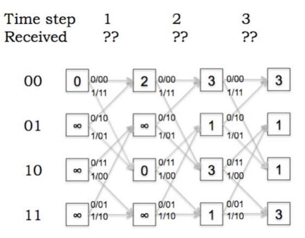
Referring to the trellis above, determine which pair(s) of parity bits could have been been received at time steps 1, 2 and 3. Briefly explain your reasoning.
