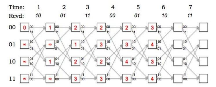
C. Fill in the path metrics in the empty boxes in the diagram above (corresponding to the Viterbi calculations for times 6 and 7).
