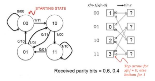
A. Complete the Viterbi step, i.e., fill in the question marks in the matrix, assuming a hard branch metric based on the Hamming distance between expected an received parity where the received voltages are digitized using a 0.5V threshold.
