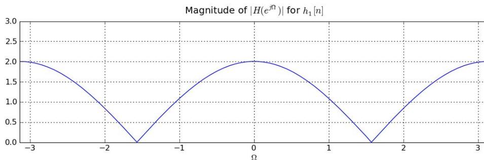
Note: the only nonzero values of unit sample response for  $H_1$  are :  $h_1[0] = 1$ ,  $h_1[1]=0$ ,  $h_1[2]=1$ .
