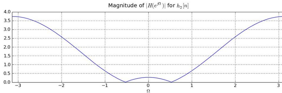
Note, the only nonzero values of unit sample response for  $H_2$  are :  $h_2[0] = 1$ ,  $h_2[1] = -\sqrt{3}$ ,  $h_2[2] = 1$ .
