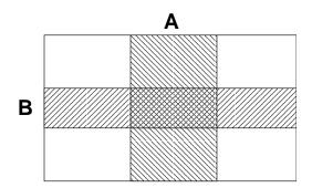
The sample space is the whole rectangle. Event *A* is a vertical stripe, and event *B* is a horizontal stripe. Assume that the probability of each event is proportional to its area in the diagram. Now if *A* covers an  $\alpha$ -fraction of the sample space, and *B* covers a  $\beta$ -fraction, then the area of the intersection region is  $\alpha \cdot \beta$ . In terms of probability:
