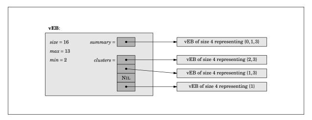
**Figure 15.2.** A vEB structure of size 16 representing the set  $\{2,3,5,7,13\} \subseteq \{0,\ldots,15\}$ .
