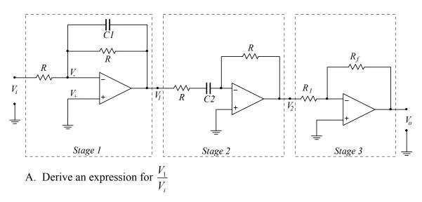
B. Derive an expression for  $\frac{V_2}{V_1}$
