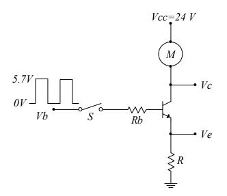
N.Rub, was careful to limit the current though the BJT by appropriately selecting resistor R and now he was ready to turn it on by closing switch S.
