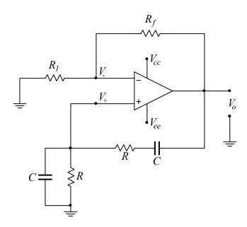
A. By considering the impedance of the elements calculate the voltage ratio  $\frac{V_+}{V_o}$
