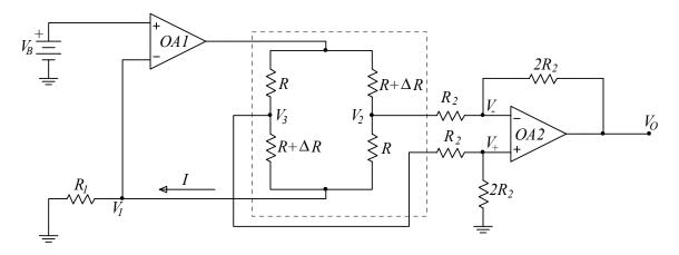
You should recognize that the resistor network enclosed by the dotted rectangle is a Wheatstone bridge. In practice such a bridge may be used in performing strain-gauge or temperature measurements.
