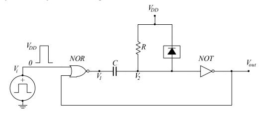
This circuit combines two logic gates (NOR and NOT) and an RC network.
