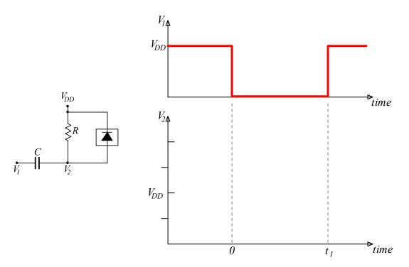
D. Now let's connect a diode to the *RC* circuit as shown below. Draw the evolution of  $V_2$  in this case.
