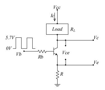
A. For Vcc=10.2 Volts, determine the value of the load resistance  $R_L$  and the emitter resistor R so that the BJT operates in the active region and the current constraint is not violated (i.e.  $Vce \ge 0.2$  Volts and  $Ic \le 50 mA$ ).
