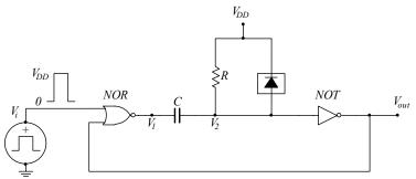
The signal  $V_i$  is a pulse as shown below. Draw the form of the voltage  $V_1$ ,  $V_2$ , and  $V_{out}$ . Indicate all relevant transition times and values.
