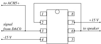
Place the device as indicated in the schematic below and make the connections shown.
