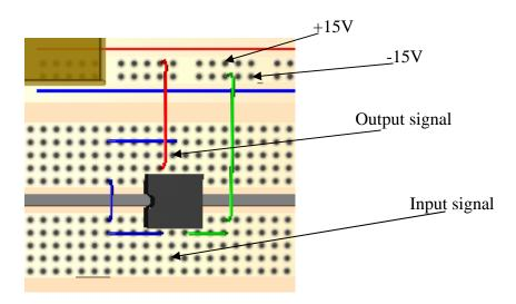
Test your circuit by connecting the power as indicated and use a 1 kHz sine wave with an amplitude of 5 Volts as the input signal.
