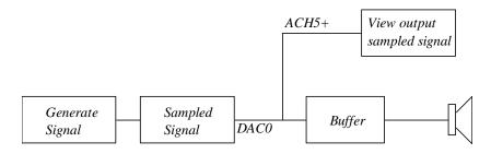
The output from the computer comes at DAC0. Connect the output signal to ACH5+. The sampled output signal appears in the lower graphs of the instrument. Notice you have to use the Start Play and Stop Play buttons in order to hear the results of your sampling selection.
