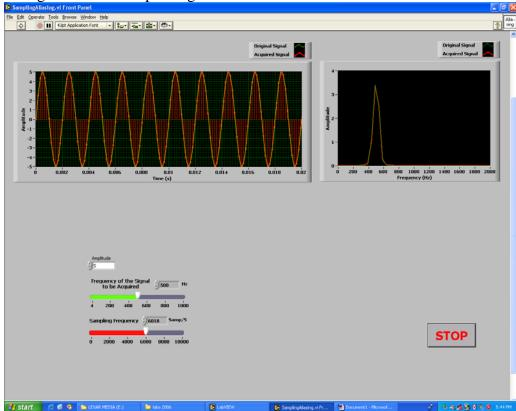
Construct a signal with a frequency of 500 Hz. Now change the sampling frequency and observe the results.
