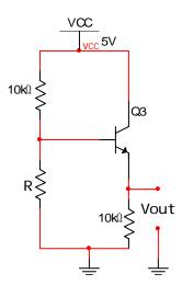
Determine the value of resistor R so that Vout = 2V
