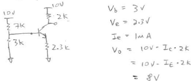
Ex: Draw  $V_o$  for  $0 < V_{IN} < 5.7V$
