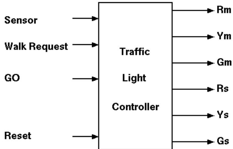
This is a conceptual developed block diagram for the machine
