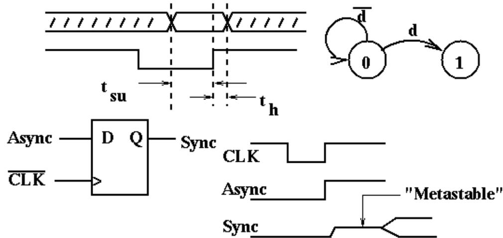
**But if inputs are synchronized according to the rule, the (single) FF will make the transition on the NEXT clock edge**
