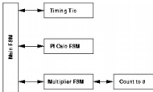
Here is my first guess at the 'Main' FSM that coordinates all. It starts other processes and waits for them to finish before going on. Note the TIC is produced by an FSM (a counter) that is NOT controlled by the main FSM.
