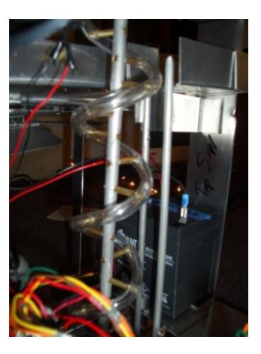
The second mechanical system was an archimedean screw. We used a single screw which trapped balls against two bars. The shaft was aluminum with 1 inch brass supports. The
