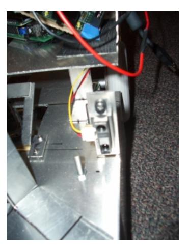
We didn't use many sensors, because we had used most of our points on the two high torque motors for our capture and elevation systems. We had two short range IR sensors on the sides of our robot. These pointed forward and were mainly used for obstacle avoidance. We also used optical encoders to help with straight driving.
