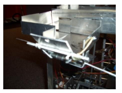
The trapdoor was the result of running out of sensor points. Ideally we would have used a servo to open and close the door. Instead, we had a mechanical system that was improvised on the last day before impounding. It was a one-shot affair, with a spring holding the door closed and a bar acting as a switch. When the bar hit a field goal upright on either side, it pulled the trap door open.
