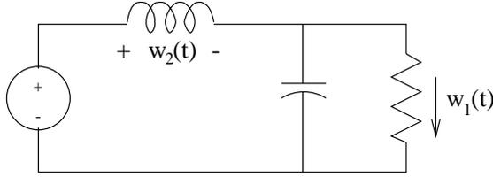
Suppose the signals (variables) of interest — the manifest signals — in the above circuit diagram are  $w_1(t)$ ,  $w_2(t)$  and  $w_3(t)$  for  $t \geq 0$ , so the signal space  $\mathbb{W}$  is  $\mathbb{R}^3$  and the time axis  $\mathbb{T}$  is  $\mathbb{R}^+$  (i.e. the interval  $[0, \infty]$ ). Picking all other component voltages and currents as latent signals, we can write the constraints that define the model as:
