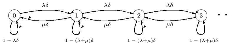
Figure 6.5: Approximating an M/M/1 queue by a sampled-time Markov chain.
