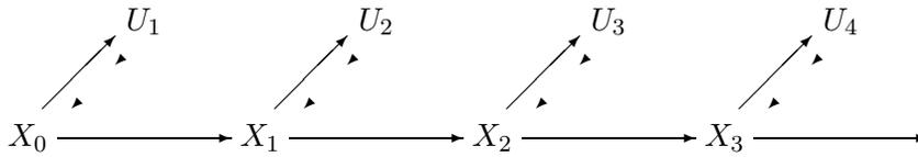
Figure 6.1: The statistical dependencies between the rv's of a Markov process. Each holding interval  $U_i$ , conditional on the current state  $X_{i-1}$ , is independent of all other states and holding intervals.
