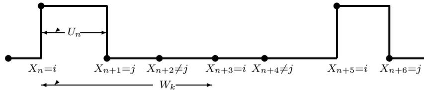
Figure 6.18: The renewal-reward process for  $i$  to  $j$  transitions. The expected value of  $U_n$  if  $X_n = i$  and  $X_{n+1} = j$  is  $\bar{U}(i, j)$  and the expected interval between entries to  $i$  is  $\bar{W}(i)$ .
