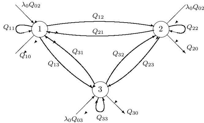
Figure 6.16: A Jackson network with 3 nodes. Given a departure from node  $i$ , the probability that departure goes to node  $j$  (or, for  $j = 0$ , departs the system) is  $Q_{ij}$ . Note that a departure from node  $i$  can re-enter node  $i$  with probability  $Q_{ii}$ . The overall exogenous arrival rate is  $\lambda_0$ , and, conditional on an arrival, the probability the arrival enters node  $i$  is  $Q_{0i}$ .
