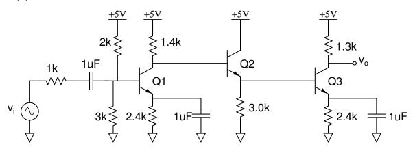
**Problem 2:** Simulate the CE-EF-CE amplifier in Circuit 1b (above) with HSPICE. Use the following data for your simulations:  $I_S = 10^{-15}$ A,  $\beta_F = 200$ ,  $V_A = 100$ ,  $\tau_F = 0.1$ ns,  $c_{jeo} = 10$ pF, and  $c_{jco} = 2$ pF. Turn in your HSPICE input file, and an Awaves plot showing the low and high frequency roll-offs.
