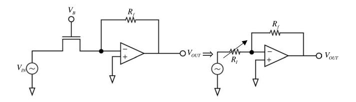
In the small-signal view of the world, the MOSFET looks like a variable resistor (if we bias things right). So the transfer function becomes
