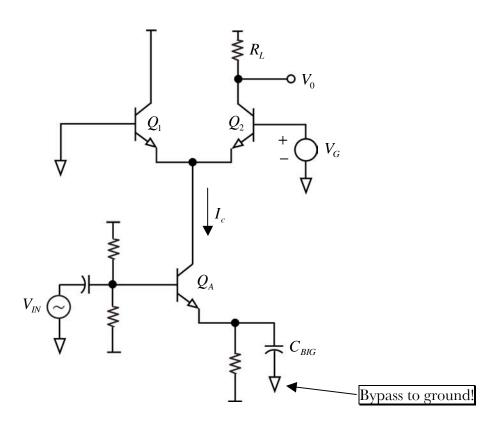
When  $V_G = 0$ , the output current from  $Q_A$  gets split evenly between  $Q_1$  and  $Q_2$  ....the gain is therefore  $\frac{1}{2}g_{mA}R_L$ , as half of the output signal current is "stolen" by  $Q_1$ . Looking in Gray and Meyer, we can find the function of  $I_C$  that actually winds up going through  $R_L$  as
