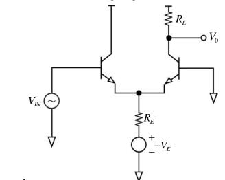
Remembering that  $g_m = \frac{qI_c}{kT}$ , derive the gain of this amplifier as a function of  $V_E$ . (Workspace)
