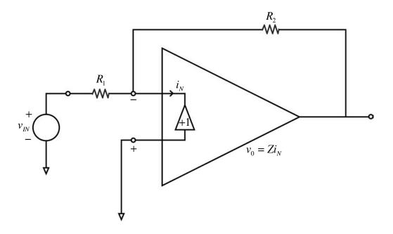
A start to the analysis is to observe that, as in the case of the voltage op-amp,  $V_+ = V_-$  (= 0). The <u>reasons</u> are different, of course. For the voltage op-amp, it was negative feedback, combined with infinite gain, that forced  $V_+ = V_-$ . Here,  $V_+ = V_-$  by construction, because we have placed a voltage buffer between them.
