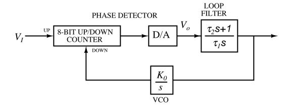
Figure 6.3: Alternative Digital Phase Detector
