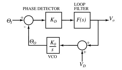
Figure 6.1: PLL block diagram
