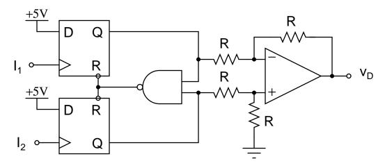
Figure 6.2: FSM phase detector
