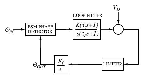
Figure 6.4: PLL block diagram
