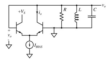
Figure 5.2: Resonant oscillator circuit
