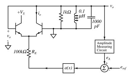
Figure 5.5: Amplitude-stabilized resonant oscillator circuit
