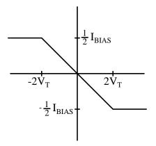
Figure 5.3: Piecewise linear I/V curve
