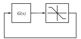
Figure 5.4: Block diagram with describing function
