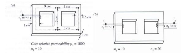
**Figure 2** (a) A single-winding magnetic circuit. (b) A coupled-winding magnetic circuit. Ferroxcube
