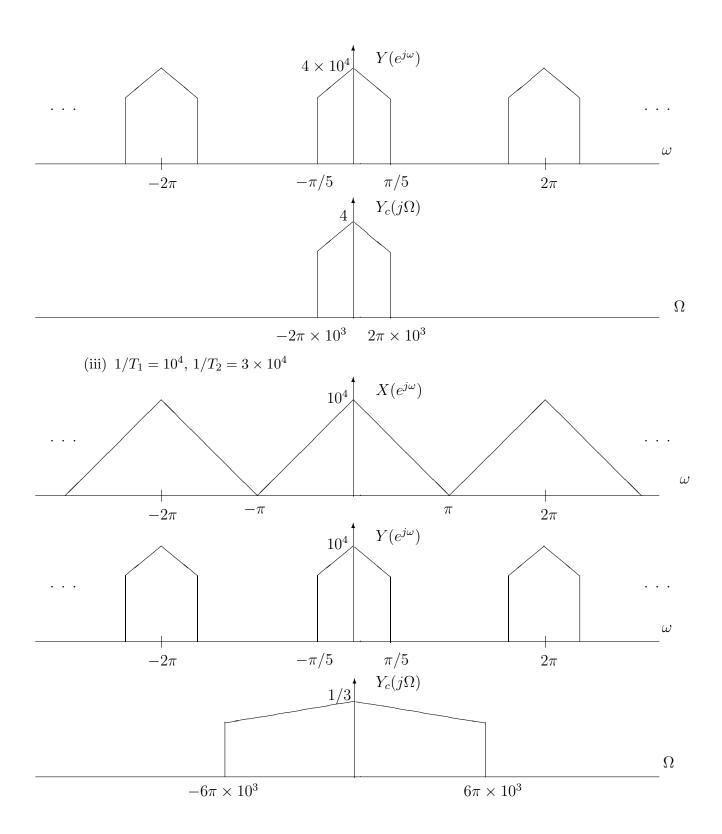
(b) From the figure below, the only portion of the spectrum which remains unaffected by the aliasing is  $|\omega| < \pi/3$ . So if we choose  $\omega_c < \pi/3$ , the overall system is LTI with a frequency response of:
