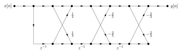
(b) Draw the lattice filter structure for the all-pole filter 1/H(z).
