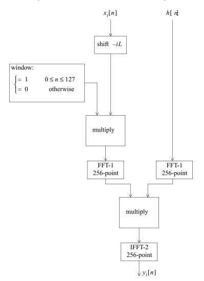
We could also use FFT-2 blocks with IFFT-1 blocks. Whichever FFT blocks are used, the signals  $x_i[n]$  and h[n] need to be zero padded to length 256 before the FFTs.
