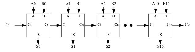
Figure 4: 16-bit ripple carry adder
