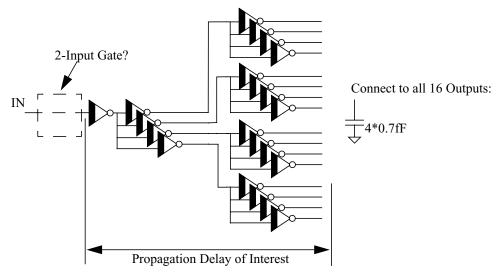
Figure 3: Sizing Sleep Device(s) for an Inverter Tree
