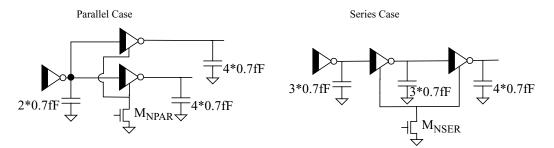
Figure 2: Sizing Sleep Devices for Parallel and Series Inverters
