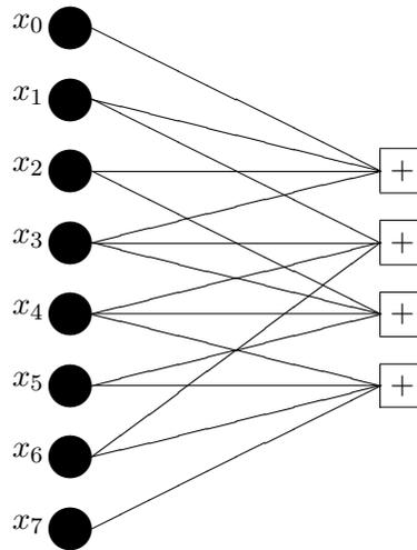
Figure 1. Tanner graph of parity-check representation for  $(8, 4, 4)$  code.
