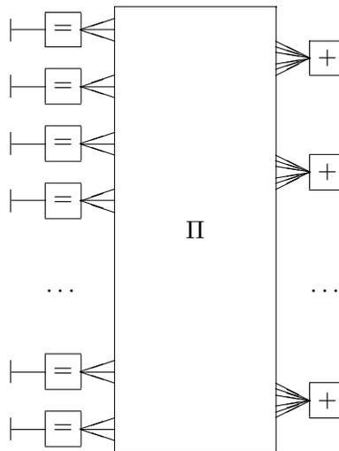
Figure 2. Normal graph of a regular  $d_\lambda = 3$ ,  $d_\rho = 6$  LDPC code.
