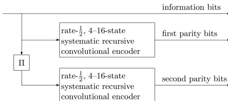
Figure 3. Rate- $\frac{1}{3}$  Berrou-type turbo code.
