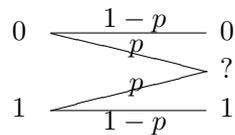
Figure 7. Transition probabilities of the binary erasure channel.
