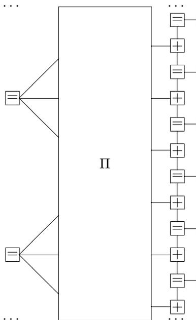
Figure 6. Normal graph of rate- $\frac{1}{3}$  RA code.
