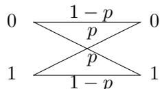
Figure 10. Transition probabilities of the binary symmetric channel.
