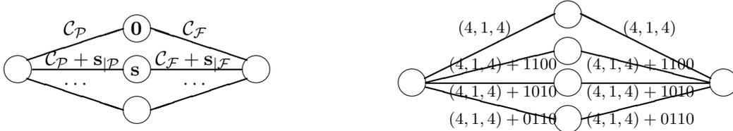
Figure 3. (a) Two-section trellis for generic code; (b) two-section trellis for  $(8, 4, 4)$  code.
