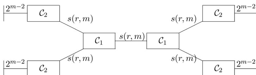
Figure 12. Tree-structured realization of  $RM(r, m)$ .
