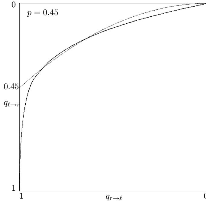
Figure 9. EXIT chart for iterative decoding of a regular  $(d_\lambda = 3, d_\rho = 6)$  LDPC code on a BEC with  $p = 0.45$ .
