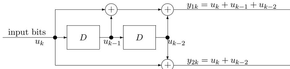
Figure 1. Four-state rate- $1/2$  binary linear convolutional encoder.
