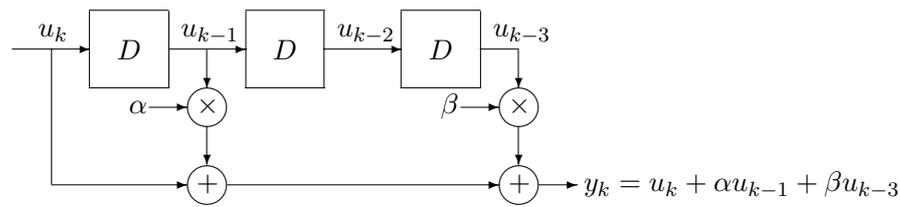
Figure 2. Realization of an LTI system with impulse response  $g(D) = 1 + \alpha D + \beta D^3$ .
