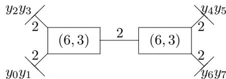
Figure 11. Tree-structured realization of (8, 4, 4) RM code.
