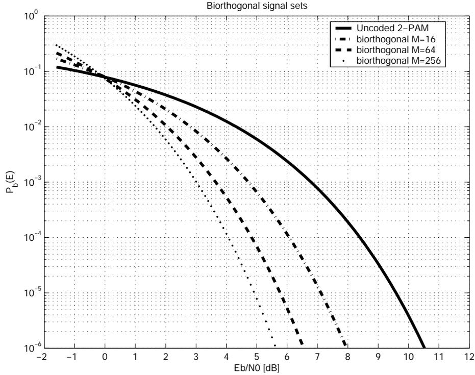
Figure 3.  $P_b(E)$  vs.  $E_b/N_0$  for biorthogonal signal sets with  $2^k = 16, 64$  and  $256$ .
