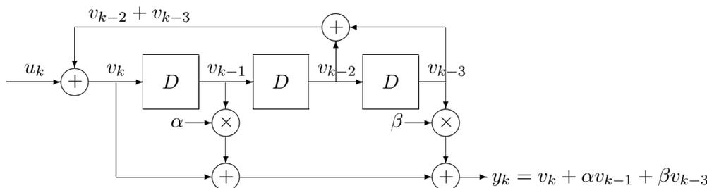
Figure 3. Realization of an LTI system with impulse response  $g(D) = (1 + \alpha D + \beta D^3)/(1 - D^2 - D^3)$ .
