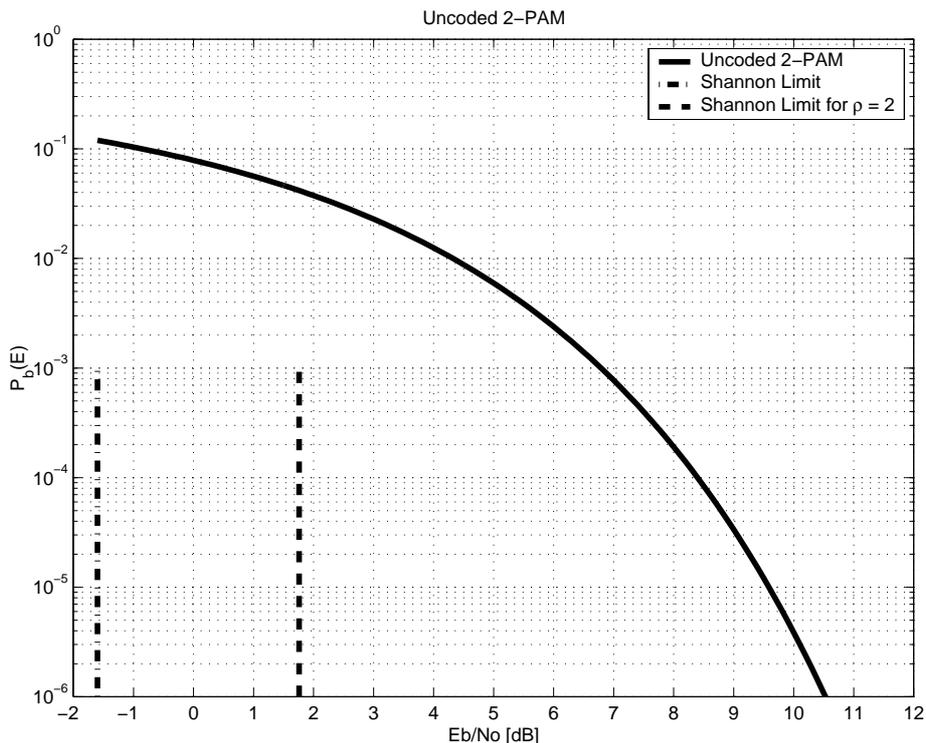
Figure 1.  $P_b(E)$  vs.  $E_b/N_0$  for uncoded binary PAM.
