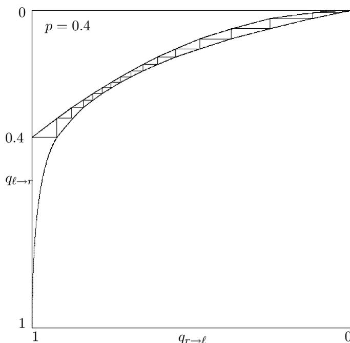
Figure 8. EXIT chart for iterative decoding of a regular ( $d_\lambda = 3, d_\rho = 6$ ) LDPC code on a BEC with  $p = 0.4$ .
