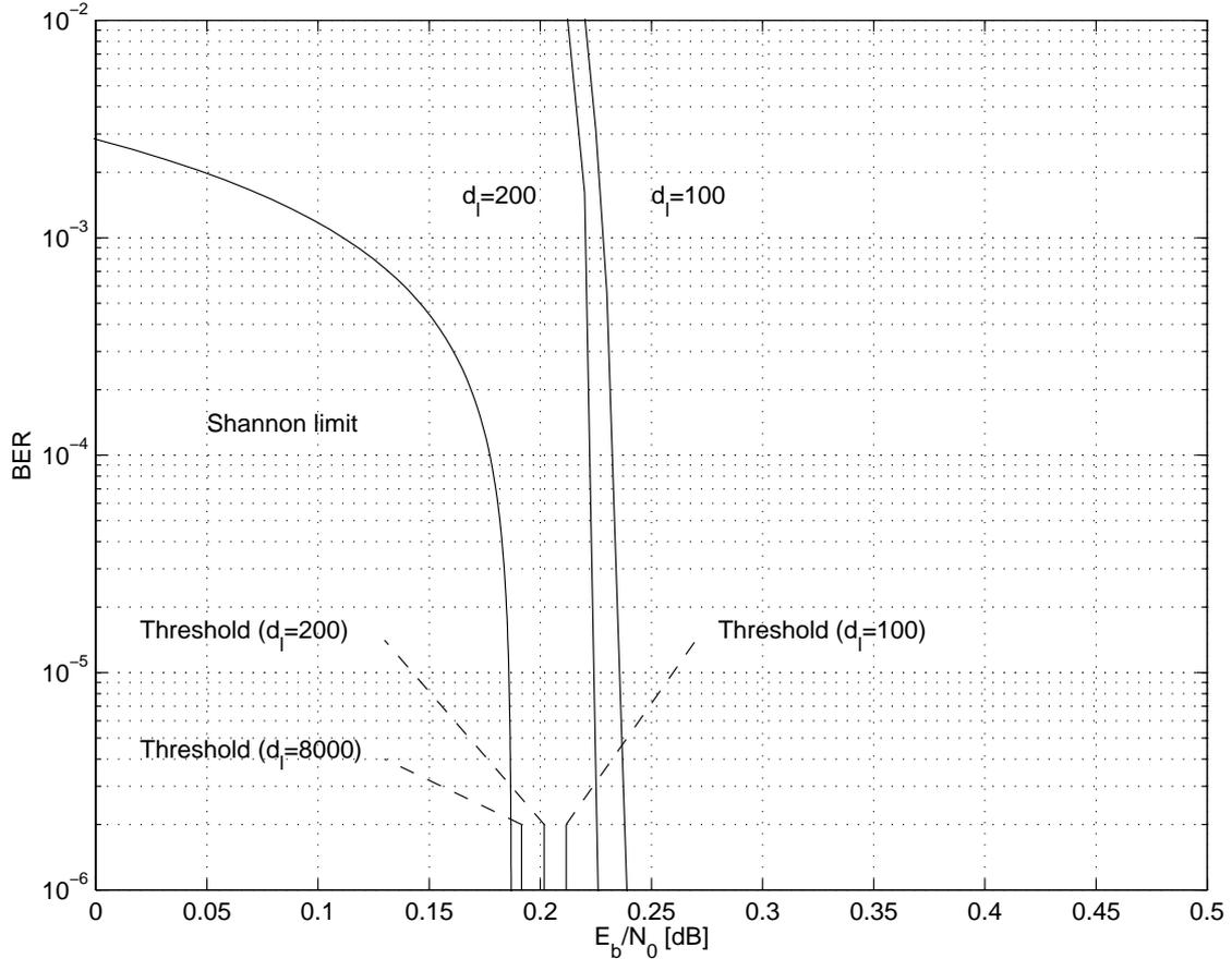
Figure 1. Bit error rate *vs.*  $E_b/N_0$  in dB for optimized irregular rate-1/2 binary LDPC codes with maximum left degree  $d_l$ . Threshold: theoretical limit as block length  $\rightarrow \infty$ . Solid curves: simulation results for block length =  $10^7$ . Shannon limit: binary codes,  $R = 1/2$ . (From [2].)
