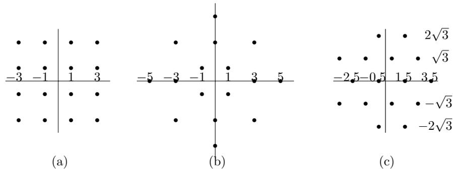
Figure 3. 16-QAM signal sets. (a)  $(4 \times 4)$ -QAM; (b) V.29; (c) hexagonal.
