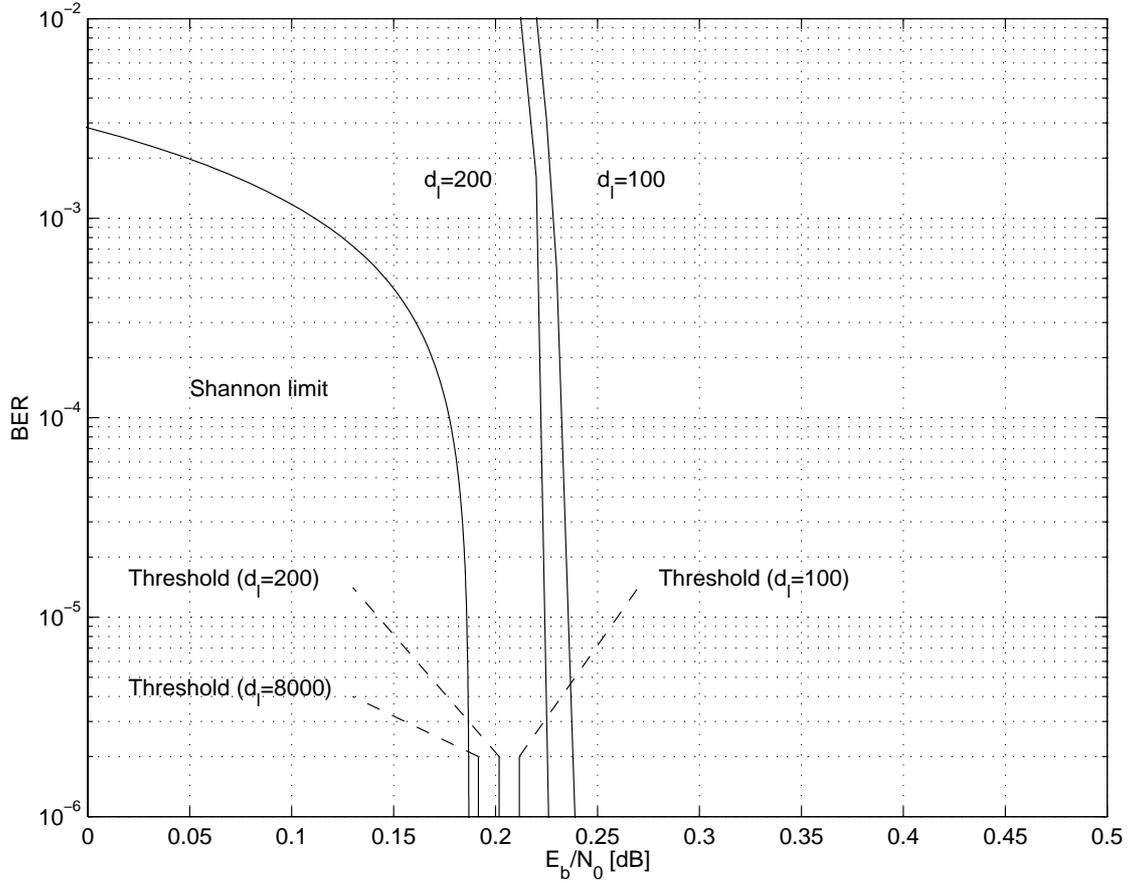
Figure 11. Asymptotic analysis with maximum left degree  $d_l = 100, 200, 8000$  and simulations with  $d_l = 100, 200$  and  $n = 10^7$  of optimized rate- $\frac{1}{2}$  irregular LDPC codes [Chung *et al.*, 2001].
