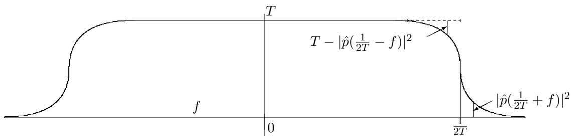
Figure 2. Raised-cosine spectrum  $\hat{g}(f) = |\hat{p}(f)|^2$  with Nyquist band-edge symmetry.
