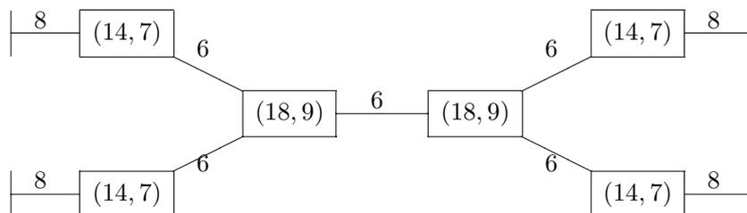
Figure 13. Tree-structured realization of  $(32, 16, 8)$  RM code.
