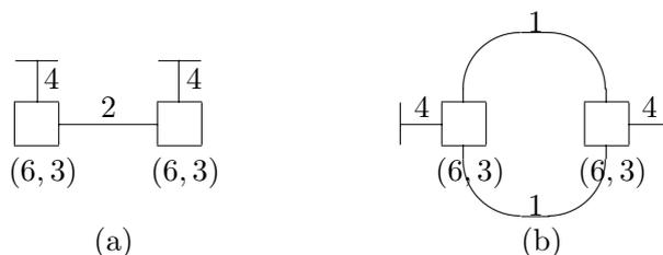
Figure 7. (a) Two-section, four-state trellis for  $(8, 4, 4)$  code;
