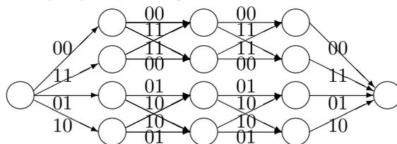
Figure 2. Four-state trellis for (8, 4, 4) Reed-Muller code.
