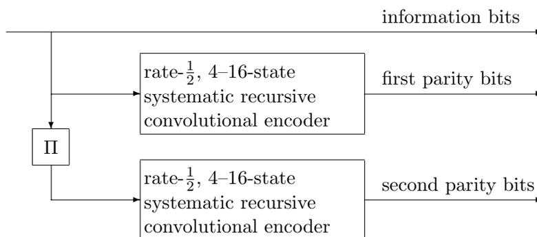
Figure 3. Rate- $\frac{1}{3}$  Berrou-type turbo code.
