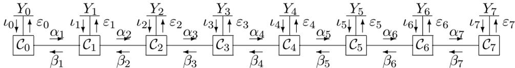
Figure 2. Flow of messages and computations in the sum-product algorithm on a trellis.
