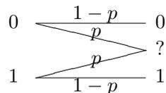
Figure 7. Transition probabilities of the binary erasure channel.
